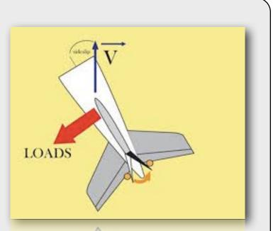
reversals are unnecessary and discouraged by pilot training programs." Current design standards do not require the airplane structure to withstand the loads that may result from such reversals, although the FAA concedes that these incidents are "low-probability events."
