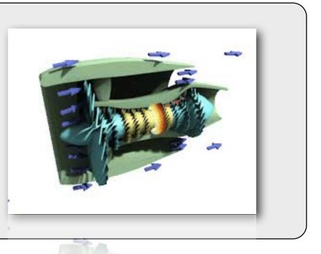
The proposed test consists of firing at the engine core the equivalent to the largest bird currently required. For departure, the test bird would be fired at 250 knots, with the mechanical engine fan speed set at the lowest expected speed when climbing through 3,000 feet agl. After bird ingestion, the proposal would require that the engine complies with post-test run-on requirements similar to those in the existing rules.
